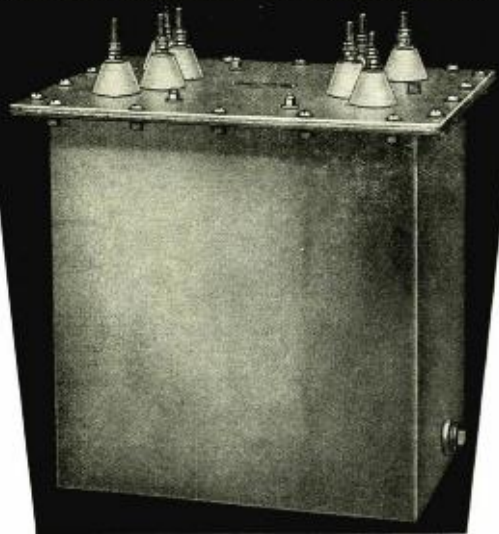
Output transformer for use between push-pull, class "B" stage using 204-type tubes and a class "C" amplifier. Operating level + 50dB; primary 1500, 1500 ohms; secondary 4750 ohms; tested at 15,000 volts; oil insulated.
